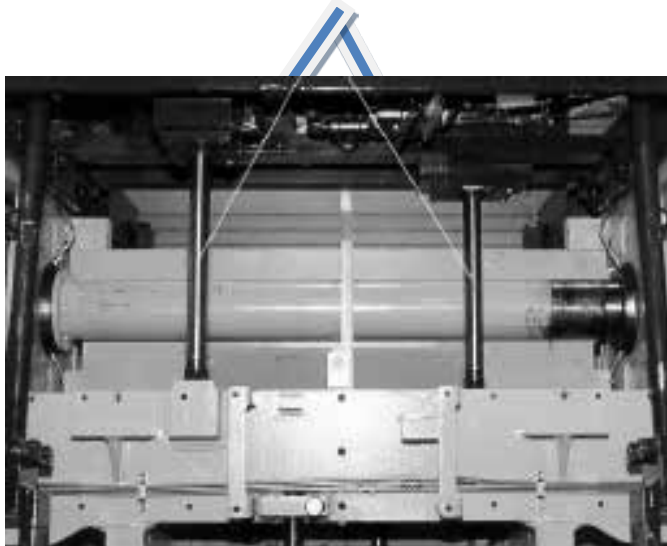
Fig. 1 - Piston rods shown in the extended position.
