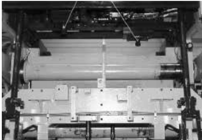
Fig. 2 - Piston rods shown in the retracted position before stripper head is in the up-stroke.
