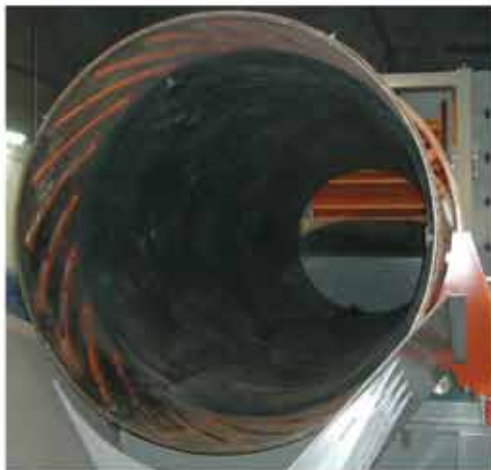
A long-life rubber lining 2" (51 mm) thick is attached to the drum with three hardened steel T-bars for straightforward, simple replacement when needed.
