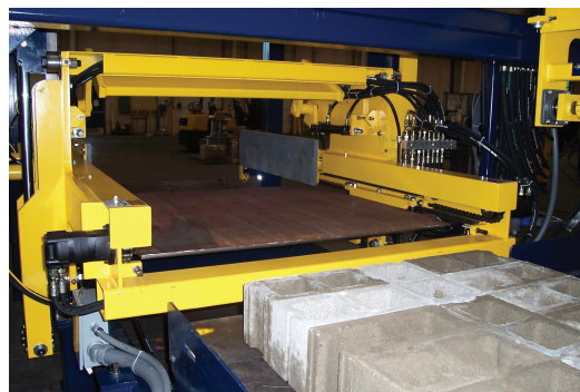
The carriage plate has dual drive motors with tapered roller bearings and sprockets located on the motor output shafts. This design requires limited maintenance.
