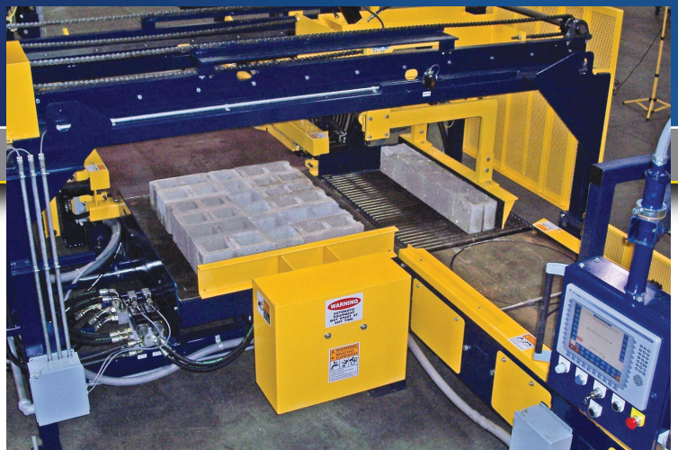
The remote panel houses the touchscreen operator interface along with the emergency stop and perimeter guarding reset
