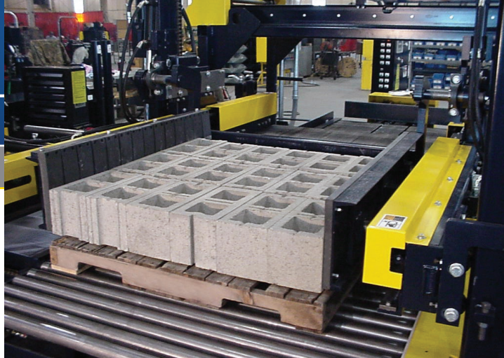
Segmented clamps provide additional control of tier placement, which is especially helpful for contoured products.
