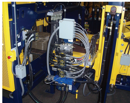
A centralized valve station provides the ability to adjust speeds from one place rather than from remote valve locations
