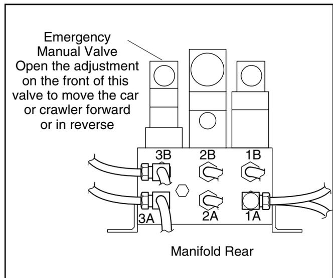
**Figure 6.4** Manifold Valves
