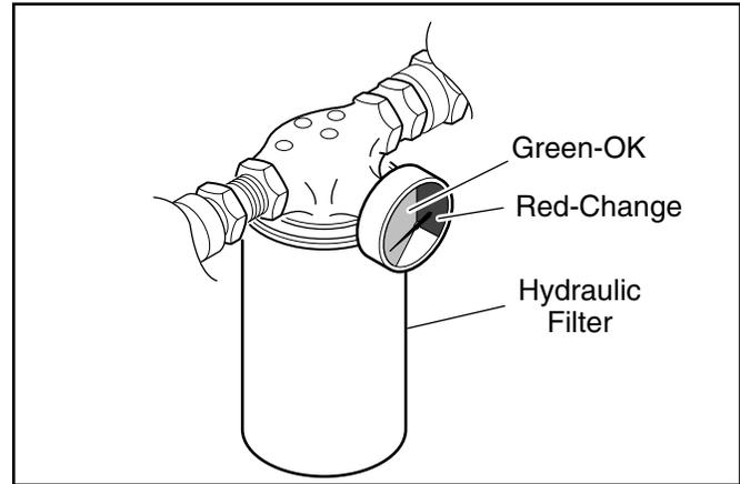
**Figure 5.11** Hydraulic Filter
