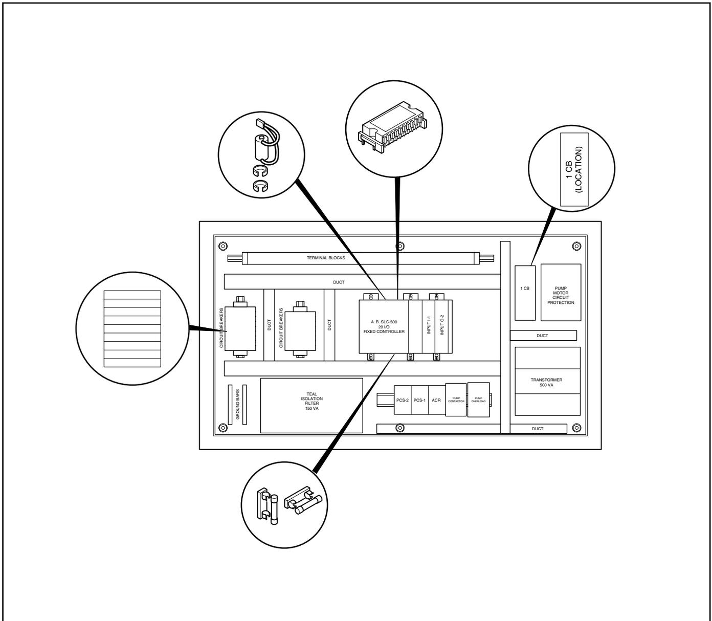
**Figure 6.2** Crawler Battery, Fuses, EPROM and Circuit Breakers
