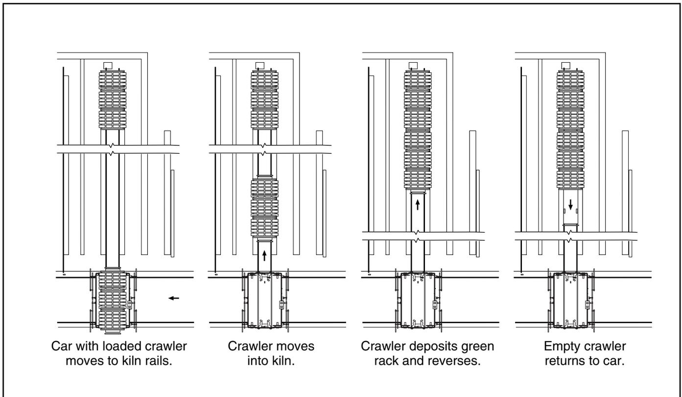
**Figure 2.3** Transporting a Green Rack to Kiln
