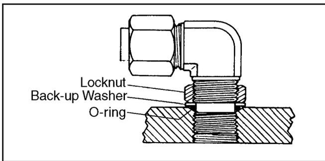
**Figure 5.6** SAE, BSPP Threads Without Check Washer
