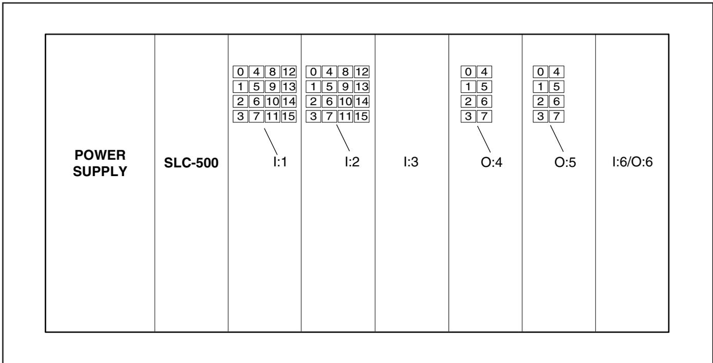
**Figure 3.17** Car Input/Output Modules
