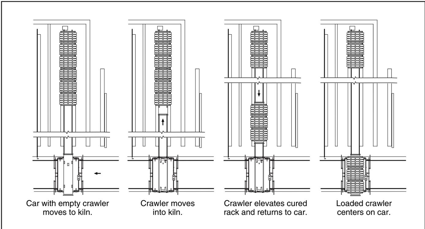
**Figure 2.4** Retrieving a Cured Rack from Storage
