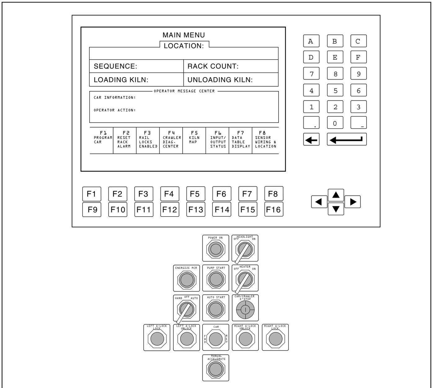
**Figure 3.1** Car Control Panel
