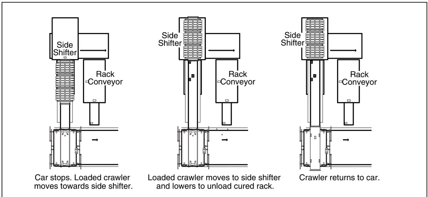
**Figure 2.1** Transporting Cured Rack to Side Shifter
