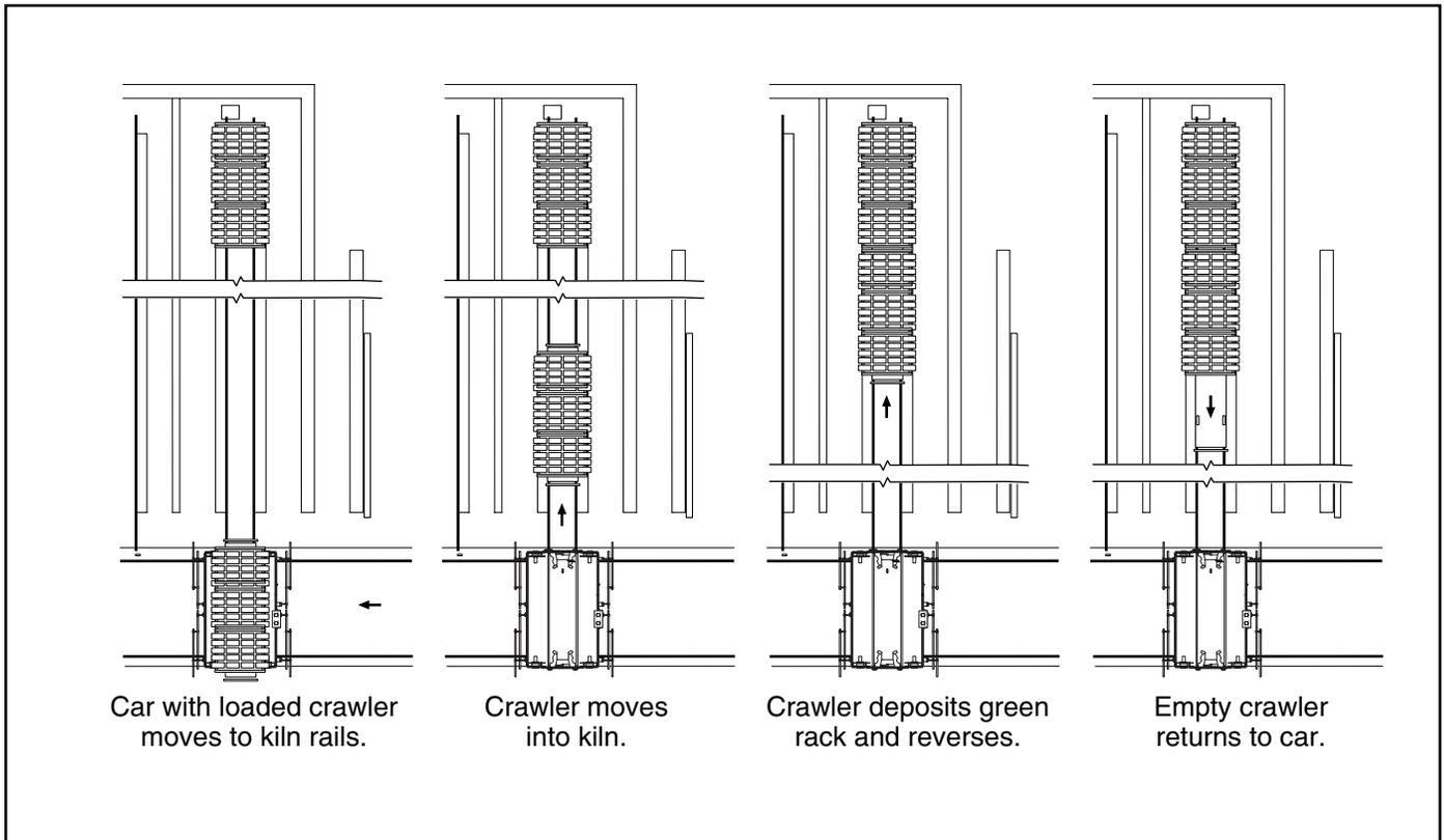
**Figure 2.7** *Transporting a Green Rack to Kiln*
