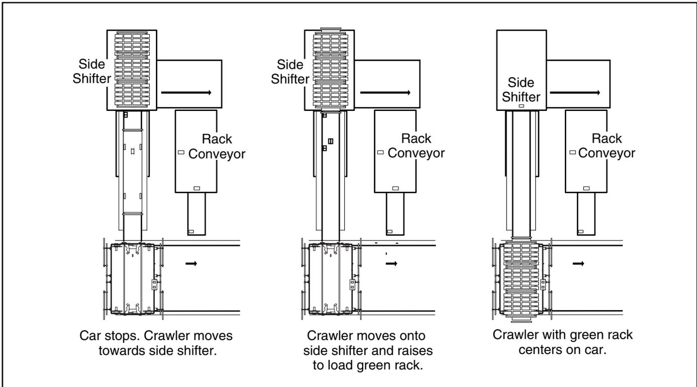
**Figure 2.6** Retrieving Green Rack from Side Shifter
