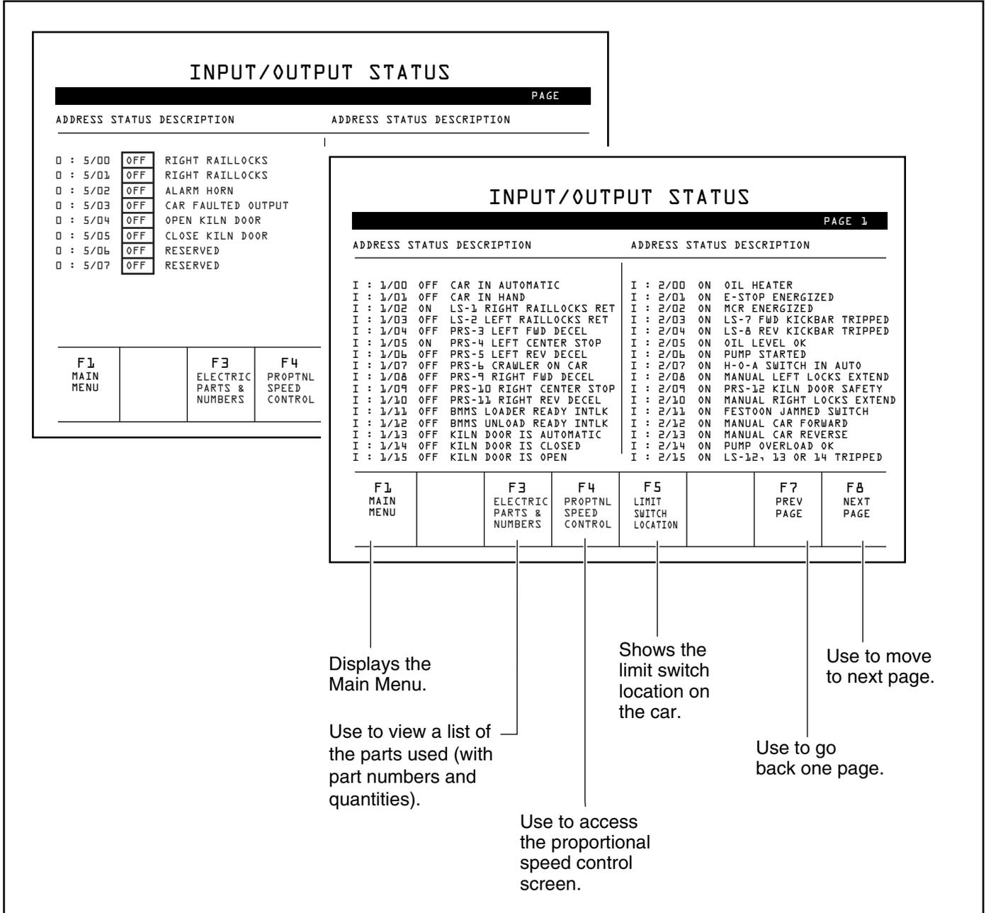
**Figure 3.13** Input/Output Status Screen
