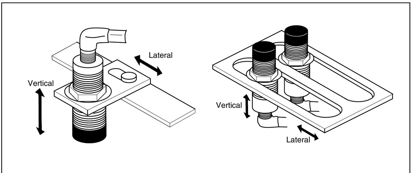
**Figure 5.1** Sensor Adjustments
