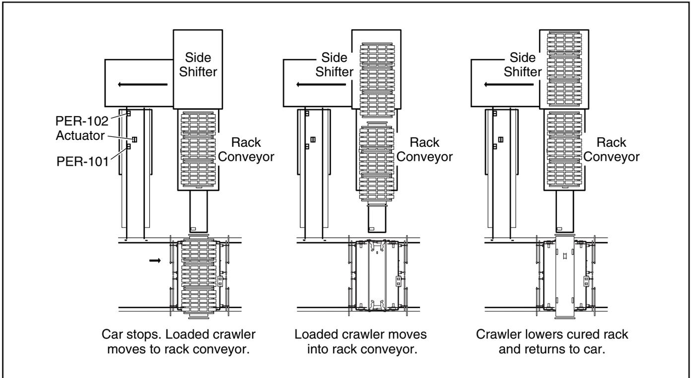
**Figure 2.5** Transporting a Cured Rack to Rack Conveyor
