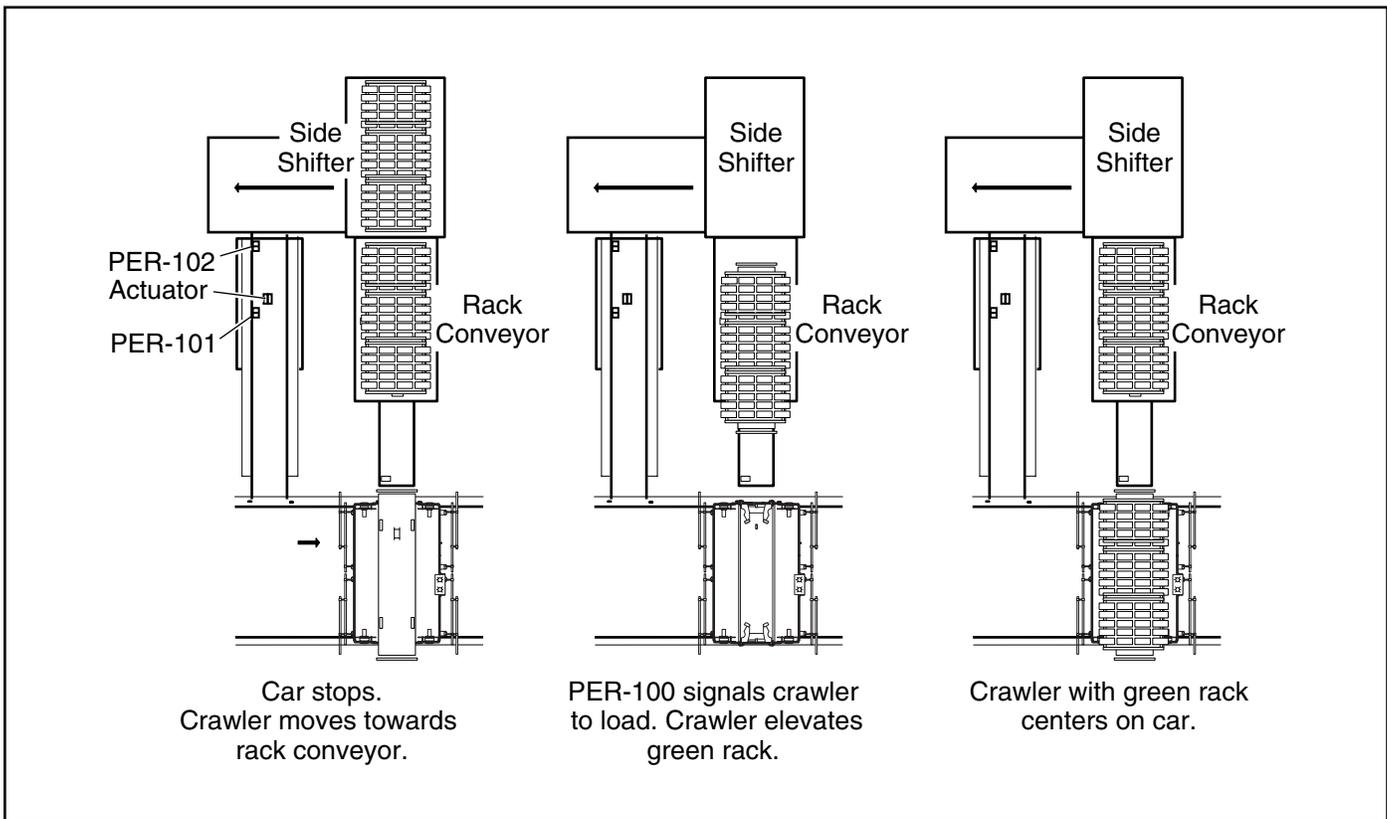
**Figure 2.2** Retrieving a Green Rack from Rack Conveyor
