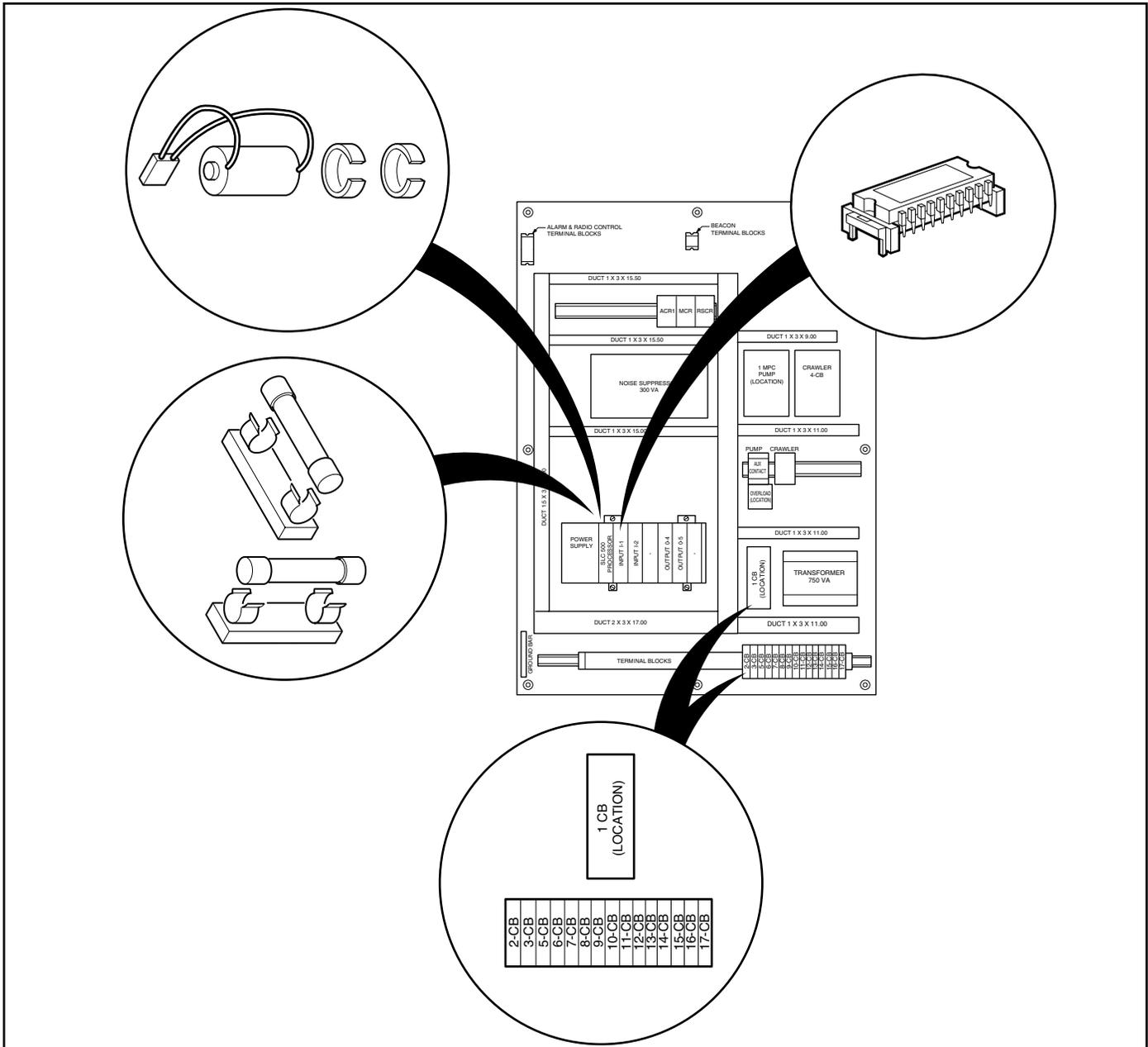
**Figure 6.1** Car Battery, Fuses, EPROM and Circuit Breakers
