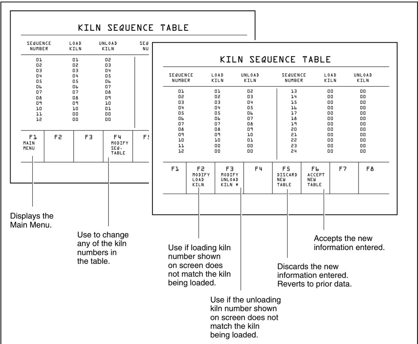
**Figure 3.9** Kiln Sequence Table Screen
