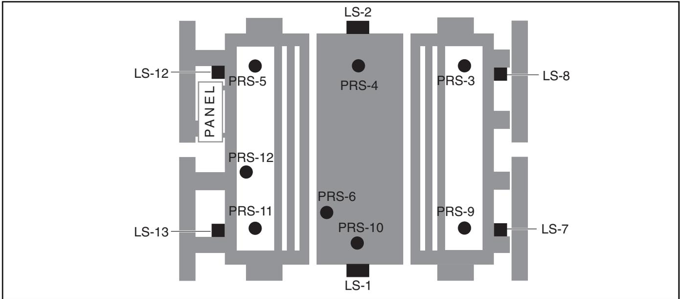
**Figure 3.12** Transfer Car Switch Locations Screen
