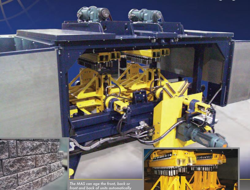
The MAS will cost-effectively expand your product line by creating unique unit faces and backs. The MAS can age segmental retaining wall units (SRWs), architectural units (split, fluted, scored, stri-face) and standard block in a wide range of sizes.
