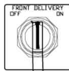
Front Delivery Conveyor ON and OFF switch.
