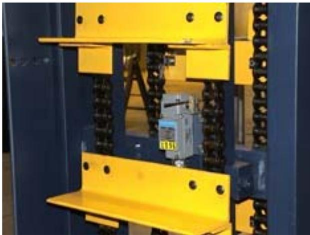
**Figure 2.3** LIMIT SWITCH PRS-1 WITHOUT GENEVA DRIVE
