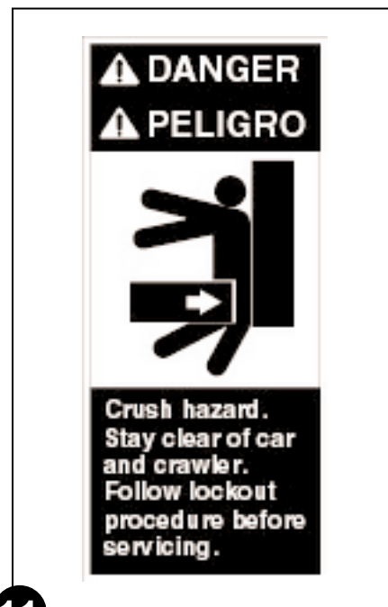
11 Vertical: 113245F0704 Horizontal: 113245F1005 Crush Hazard Vertical: Width 4 1/8 inch Vertical: Height 7 inch Horizontal: Width 10 inch Horizontal: Height 5 3/4 inch
