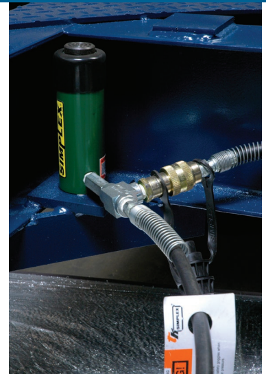
This close-up view shows the standard hydraulic strip assist feature supplied for the solid tapered cores
