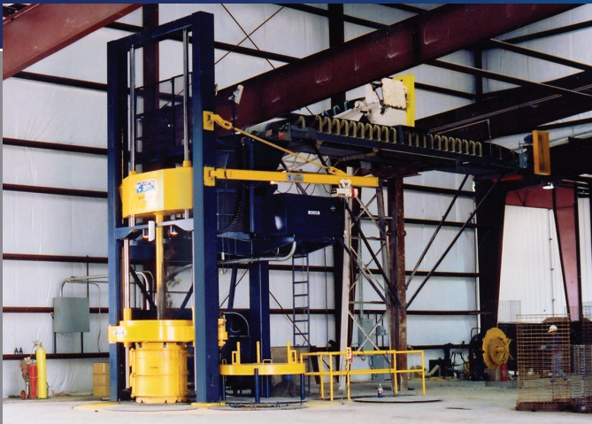
Side view of the Model A-60 Advantage machine illustrating the unique three-post frame configuration. This design allows material to be fed into the holding hopper from the rear (as shown here) or either side.
