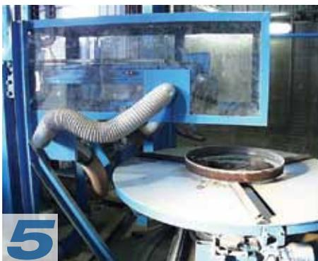
Once the pallet and/or top header ring has been removed from the pipe, it moves on a table to the cleaning station where it rotates as wire brushes clean its surface.
