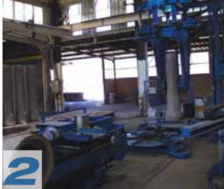
After the cured pipe is moved to the depalletizer, the pallet is removed by pneumatic devices.
