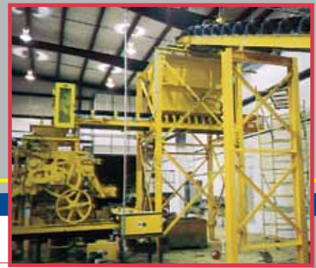
Independent metering hopper with metering conveyor feeding the block machine
