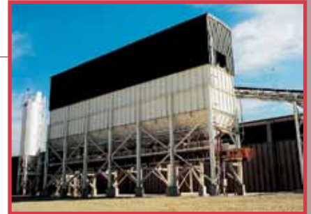
Six W-2000 model aggregate bins with 30" X 72' (750 mm x 21,600 mm) weigh belt conveyor
