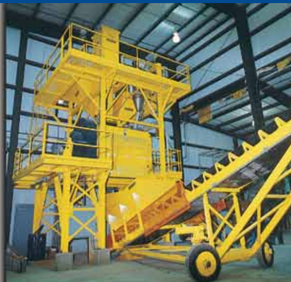
Besser batch mixer with aggregate holding hopper, cement batcher and radial metering conveyor
