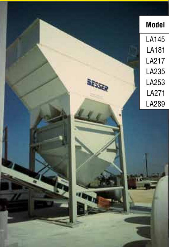
Weigh hopper under "LA" style aggregate
