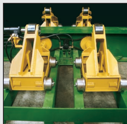
Hydraulic roll positioner is particularly useful in helping load, unload, center and rotate large-diameter pipe.
