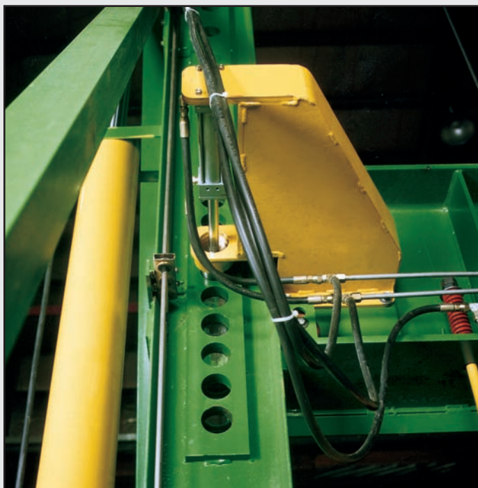
Automatic pin positioner, which inserts and removes the loading beam pins without operator assistance, is operated from the weatherproof control console.
