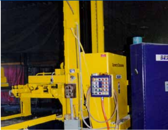
Enlarged view of E-Model Besser-Matic, showing the control station and panel.
