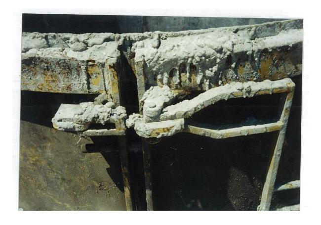
Concrete build up can misalign, twist and warp forms. Forms that are out of shape produce inferior products
