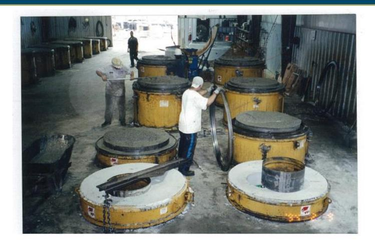
Forms can provide 25 or more years of service with proper maintenance and adjustments
