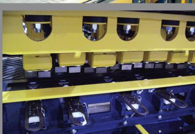
The Stone Aging Machine (SAM) gives concrete paving stone an aged appearance. The SAM utilizes product tilting zones and oscillating heads that propel loose-fitting impactors against the pavers. Impacting is totally random and is adjustable so that different aged looks can be achieved. The SAM is versatile and can be used inline or out-of-line.
