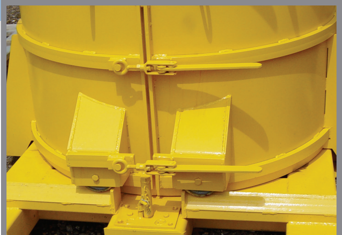
The roll-back wheel assemblies and actuator
