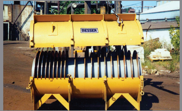
Grade ring battery form sets, in this instance incorporating a two-piece jacket, will produce multiple grade ring sections from a single pour
