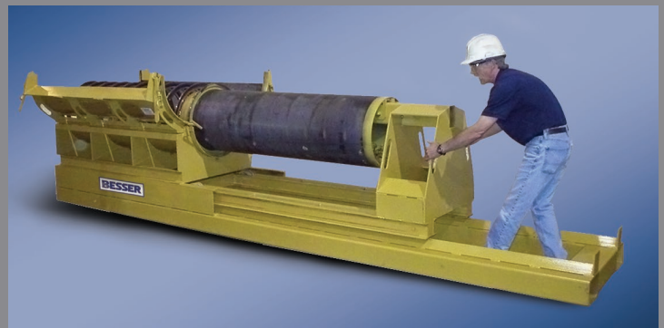
Product setup and stripping is simplified as only one production employee is needed to roll the collapsible core in and out of the form
