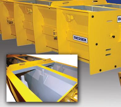
The Besser line of heavy duty wet cast median barrier form equipment is engineered and built with the features precasters need to profitably pour quality products. Median barriers are poured upside down for best finish.
