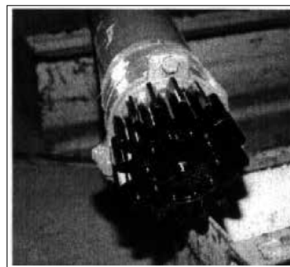
Fig. 3 - View of new pinion with the new locking assembly.
