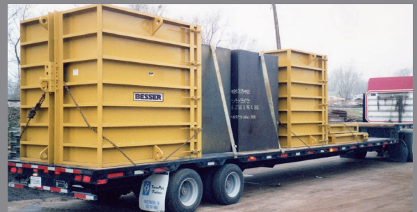
Rugged form sets are built from heavy steel plate with channel rib reinforcing for strength and reliability, as seen on these two-piece jackets, collapsible cores and lid forms
