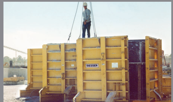
Preparing to strip utility box products from rollback jackets with air-assist collapsible cores
