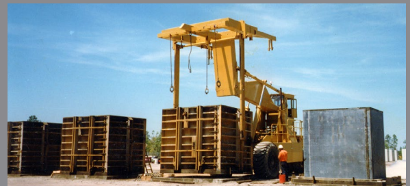
Utility box production line using 114" x 92" x 114" (2900 mm x 2300 mm x 2900 mm) two-piece outer jackets and manually operated collapsible cores
