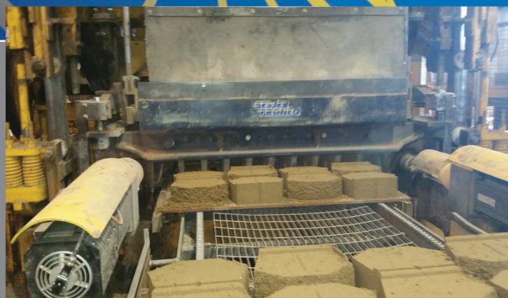
The Superpac® production rate is impressive – producing up to 3240 8" x 8" x 16" (200 mm x 200 mm x 400 mm) units an hour.
