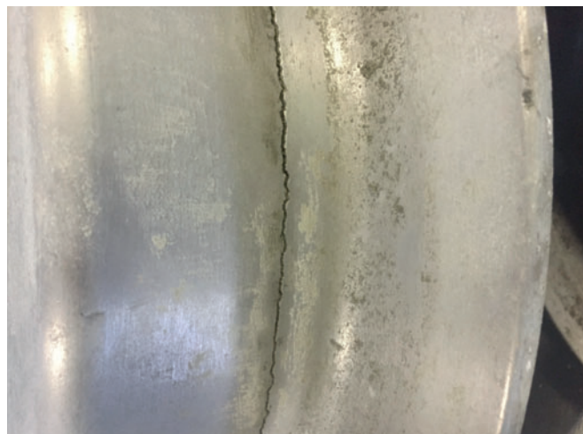
The pallet is broken and out of tolerance. Don't use this pallet!
