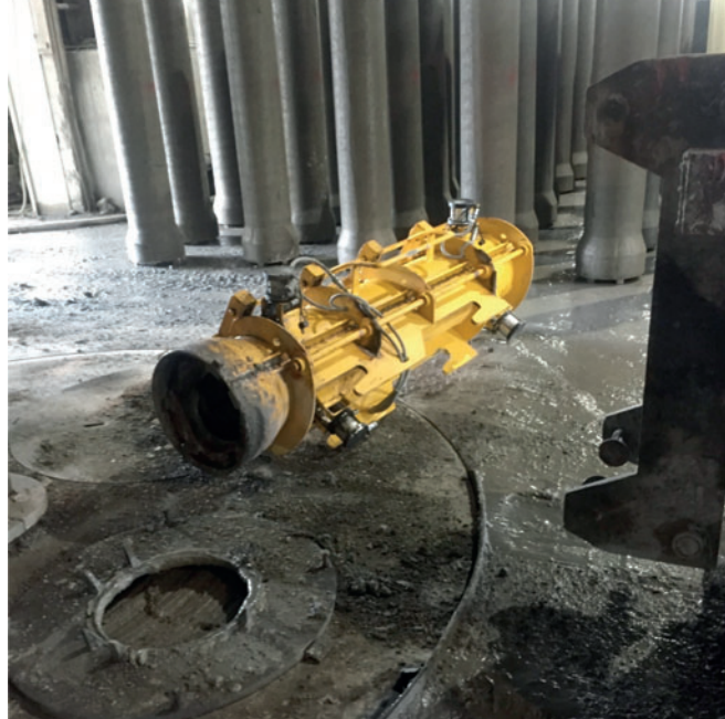
This mold was dropped. It must be checked for damage before using.
