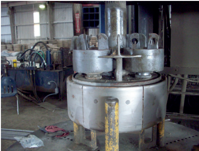
This packerhead is severely worn. The rollers, bearings, tops, hoods, wear bands and segments all must be replaced.
