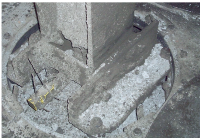
This broken switch and table race are covered in 17" of concrete, making it extremely difficult to access them. It is critical to keep your plant clean and fix equipment
