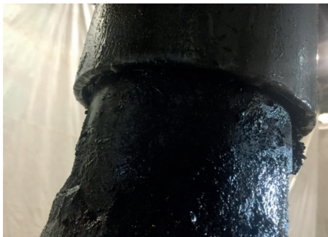
This bushing is worn. It needs to be replaced and a new one aligned in the machine.
