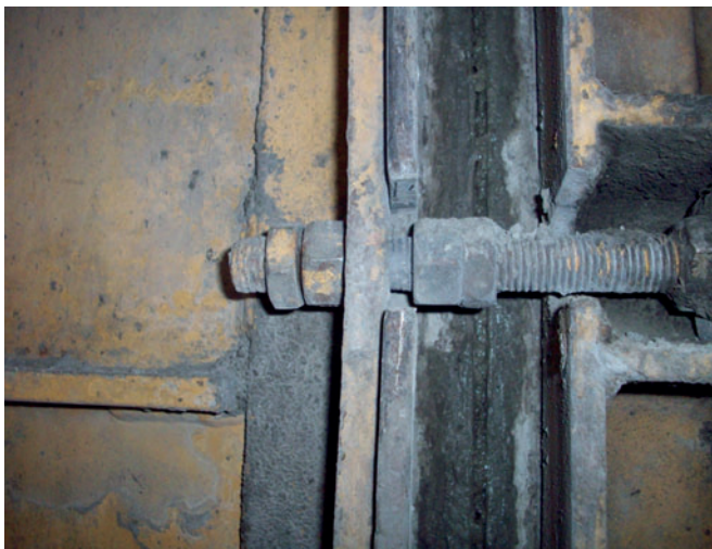
Bent lock and latch with open mold seam latched. This must be repaired to avoid wear.
