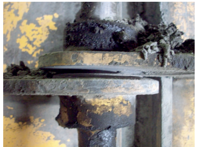
There should be grease here. The hinges are bent and worn.
