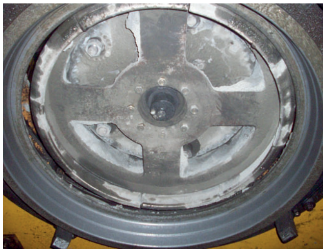
The compacted LB frame is out of balance; to remain in balance it must be cleaned daily.
