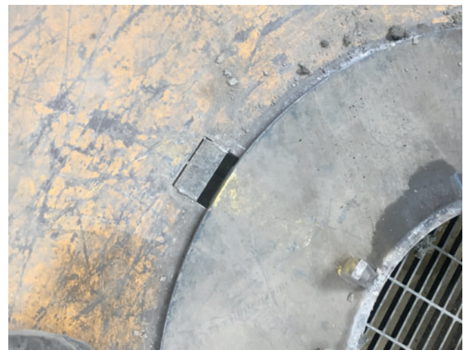
Loose table hardware allows the plate to shift. The tolerance for alignment is 1/32"; this one is off by 1/2".
