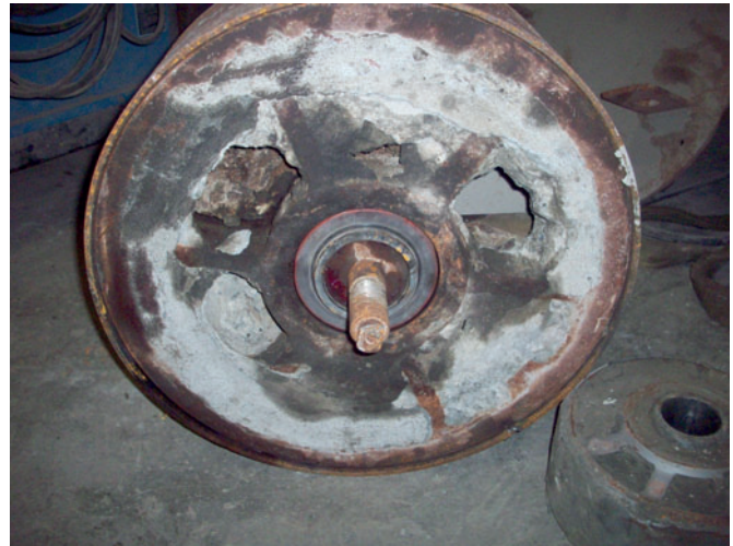
The compacted rollers are out of balance. They must be cleaned and filled with foam.
