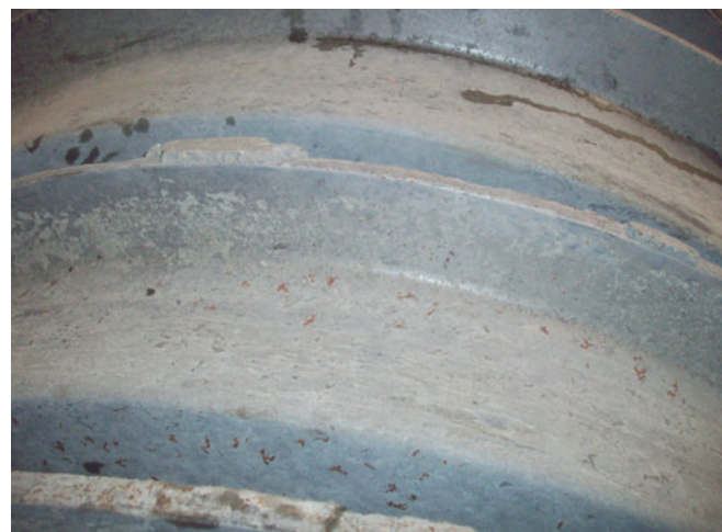
Dirty OD of the pallet will cause excessive mold wear and bad bells. Pallets MUST be cleaned daily.
