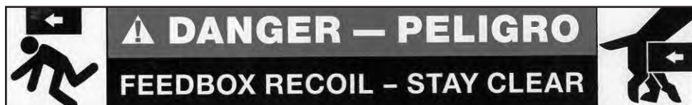
01999-400082 Crush Hazard Width 6-1/4" Height 9-1/2"
