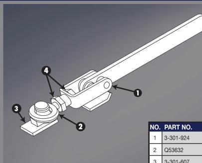
PART NO. 3-301-925 (complete JL-500S assembly) PART NO. 3-301-925A (less trunnion)
