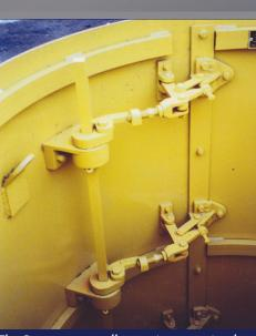
The Besser core collapser is recognized throughout the precast industry for its simplicity, durability and efficiency
