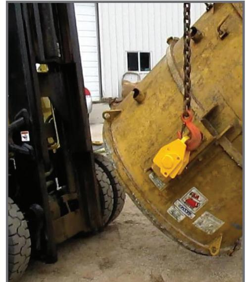
*The new brake device reduces the dangerous swinging motion by 85 - 90% when the form is rolled over.*
