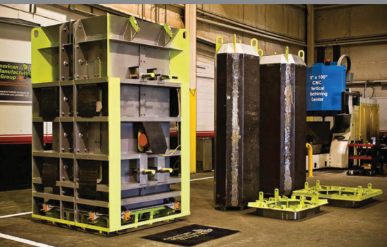
A typical example of a rise adjustable form and solid cores for dry cast egg laying
