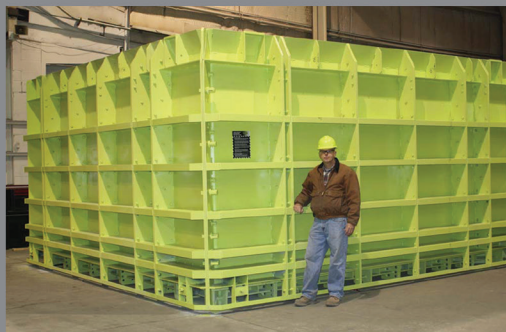
Besser manufactures several variations of adjustable box culvert mold equipment. The wet cast mold construction shown here is similar to static cast or egg lay mold construction.
