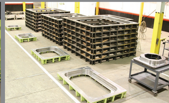
Besser adjustable pallet assemblies 4' x 2' through 8' x 8' for rubber gasket joints
