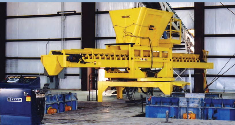
156" (4000 mm) Vibro-Mac with the computerized tracking option producing box culvert sections. This particular model features a flat shuttle-style system and provides computerized tracking for feeding various round and non-round pipe and box culvert profiles.
