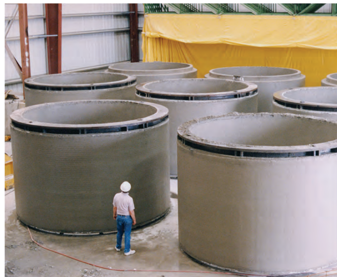
A kiln containing 144" x 8' (3600 mm x 2.5 m) Vibro-Mac produced product. Each piece has a 13" (330 mm) wall thickness and weighs 54,000 pounds (24,494 kg).
