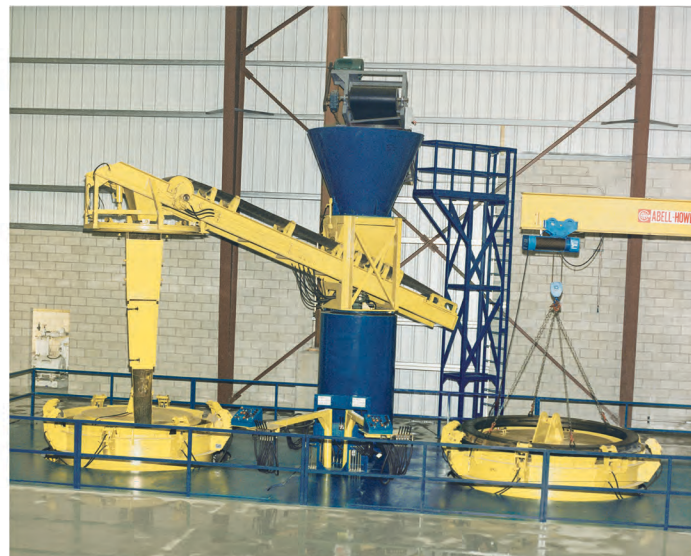
The 156" (4000 mm) model Vibro-Mac machine (pit installation) producing 144" x 8' (3600 mm x 2.5 m) pipe on the right station and 102" x 8' (2600 mm x 2.5 m) pipe on the left station.
