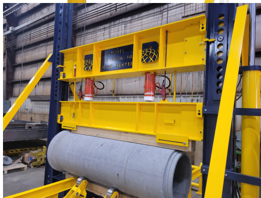
A hydraulic lift cylinder raises and lowers the loading beam. The heavy-duty rams are mounted upside down to keep water out of the cylinder and assures accurate testing.
