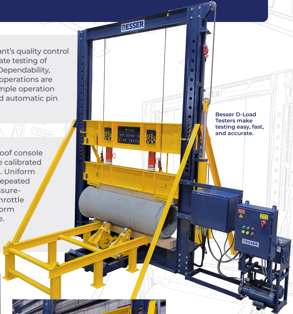
A hydraulic lift cylinder raises and lowers the loading beam. The heavy-duty rams are mounted upside down to keep water out of the cylinder and assures accurate testing.
