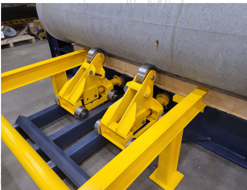
The hydraulic roll positioner centers and rotates pipe into position for testing.
