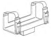
Spacer Block, bench vise supports vibrator shaft when shaft is clamped in vise.
