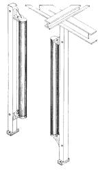
Pallet guide rollers are designed to guide loaded pallets into the rack bay. The rollers effectively align pallets without damaging "green" block and help eliminate unnecessary downtime from jammed pallets. These rollers are engineered for easy installation.
