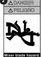
Close front panel and stay clear during operation. Follow lockout procedure before servicing.
