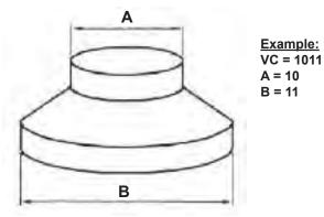
These vinyl connectors help to contain dust within charging systems and prevent water damage to cement batchers.
