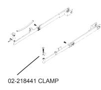
This design of grid support bars bolt together to facilitate replacement of worn front sections. Right hand and left hand pieces are no longer required because parts interchange from side to side. Front sections are hardened to resist wear. New front grid clamp blocks are included with the set of parts.
