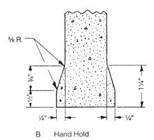
Hand hold is optional on 2 and 3 core block. Dimensions of units: In practice, the first dimension of a concrete masonry unit represents the thickness; the second dimension, the height, the third, length.
