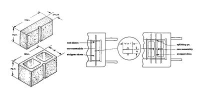
NOTE: 3-5/8", 5-5/8", 7-5/8", 9-5/8" or 11-5/8" W x 15-5/8" L compartment. New or reworked mold top plate and cutoff parts and new or reworked plungers may be necessary. This can be done in metric as well, 190 mm wide becomes 196.5 mm wide.
