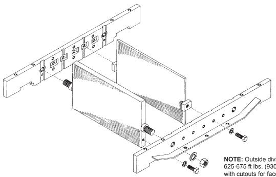
**NOTE:** Outside division plates should be torqued to 625-675 ft lbs, (930-1005 nm). Outside division plates with cutouts for face liners should be torqued to 175-195 ft lbs, (260-290 nm).
