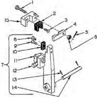
NOTE: 02-645856 SOP to install mold lock assembly on machines using pin type mold guidance.
