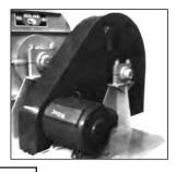
NOTE: BESSER RECOMMENDS REPLACING EXPANDED METAL GUARDS WITH GUARDS CONSTRUCTED OF SHEET METAL.
