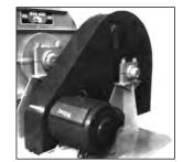
NOTE: BESSER RECOMMENDS REPLACING EXPANDED METAL GUARDS WITH GUARDS CONSTRUCTED OF SHEET METAL.
